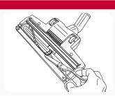
Lay the Turbobrush on a flat surface and turn over to expose the brushbar. Using a pair of scissors, cut through any threads or hairs caught by the brushbar that have wrapped around the guides.
