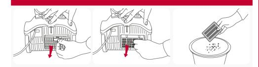
Post-motor filter is located in the right side wheel. Hold the centre of the wheel and twist wheel cover anti-clockwise. With the wheel cover off the post-motor filter is easily removed.
