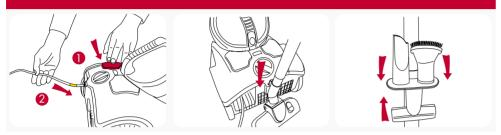
**NOTE:** For convenience there is a parking slot located at the rear of the vacuum cleaner where the floor head and tubes can be attached for storage and carrying.
