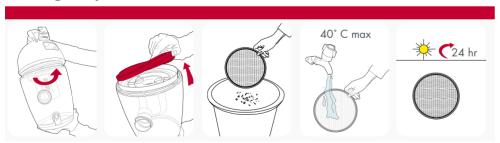
Wash filters with warm water (40°C MAX) at least every 3 months for best cleaning results. Do not use the vacuum cleaner without all of the filters in place.
