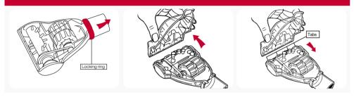
Turn the TurboTool over and slide Detach lower housing and off the locking ring.
