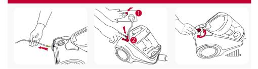
**NOTE:** Fully unwind the power cord. A yellow mark on the cord indicates the recommended cord length. Do not exceed the cord length beyond the vellow mark.
