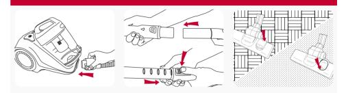
NOTE: The Turbobrush, hard floor tool, crevice tool, upholstery tool and dusting brush can all be attached directly to the telescopic tube or hose handle. The TurboTool should first be attached to the supplied connector before fitting onto the hose handle.
