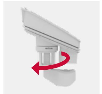
Twist the separator clockwise to release from the lid.
