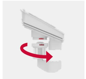
To re-fit, line up the separator tab with the lid tab and twist anticlockwise to lock.
