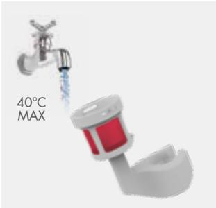
Wash the separator mesh under running water (40° max) to remove any dirt and debris.
