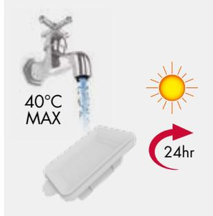
Wash the filter under running water (40°C max). Leave for at least 24hrs or until fully dry before replacing.
